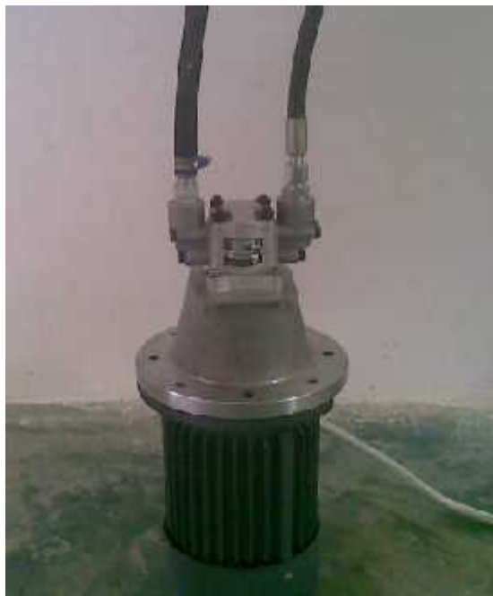
Figure 4.4 Gear pump and electrical motor
