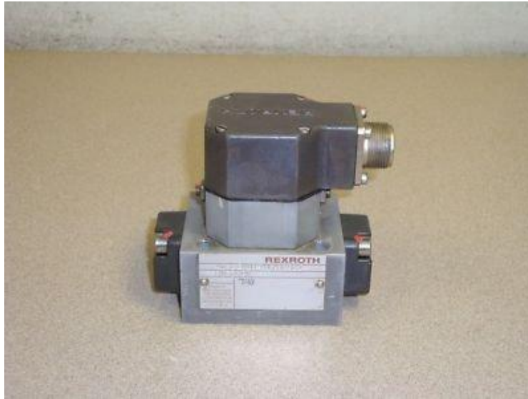
Figure 2.13: Single-stage servo valve with electrical position feedback.
