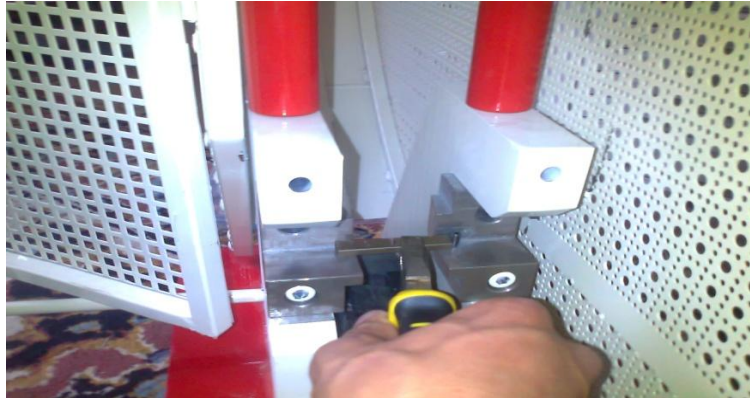
Figure (5.5): Install specimen in impact machine.
