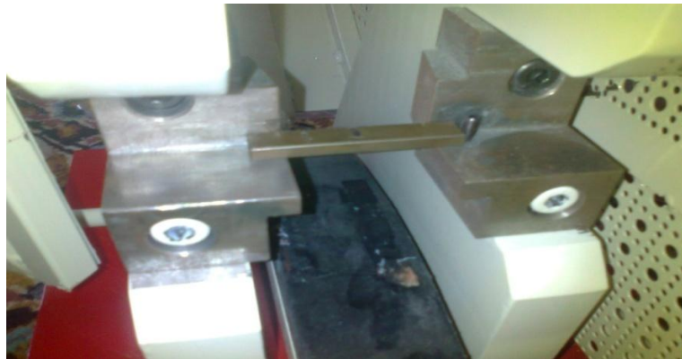
Figure (5.1): Suitable way to install specimen .
