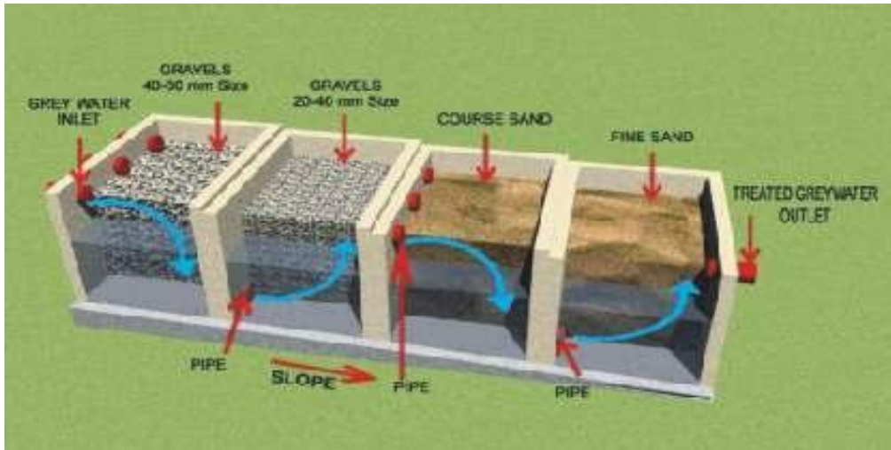
Figure 4 : Up flow Down flow Filter
