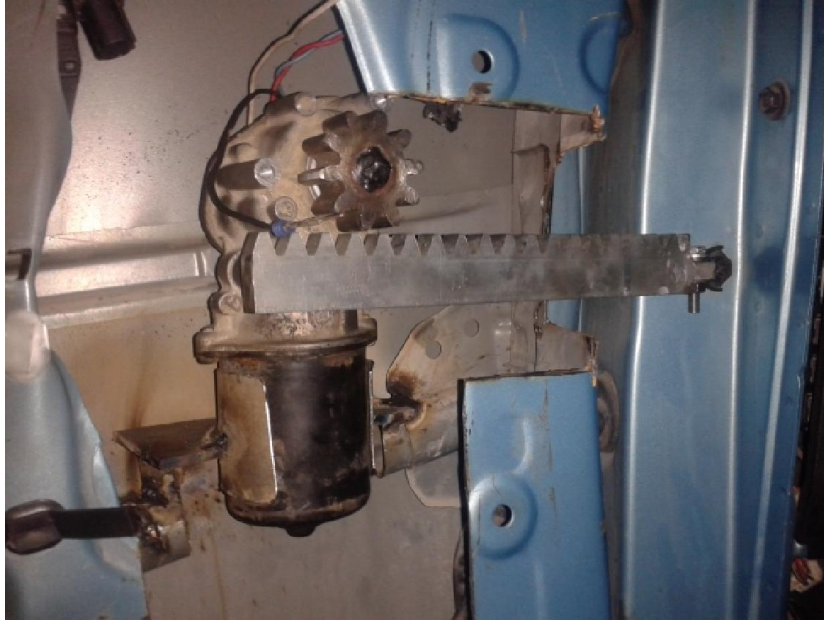
Figure (4.5): The Electrical doors design
