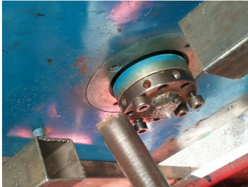
Figure (5-10):Broken shaft
