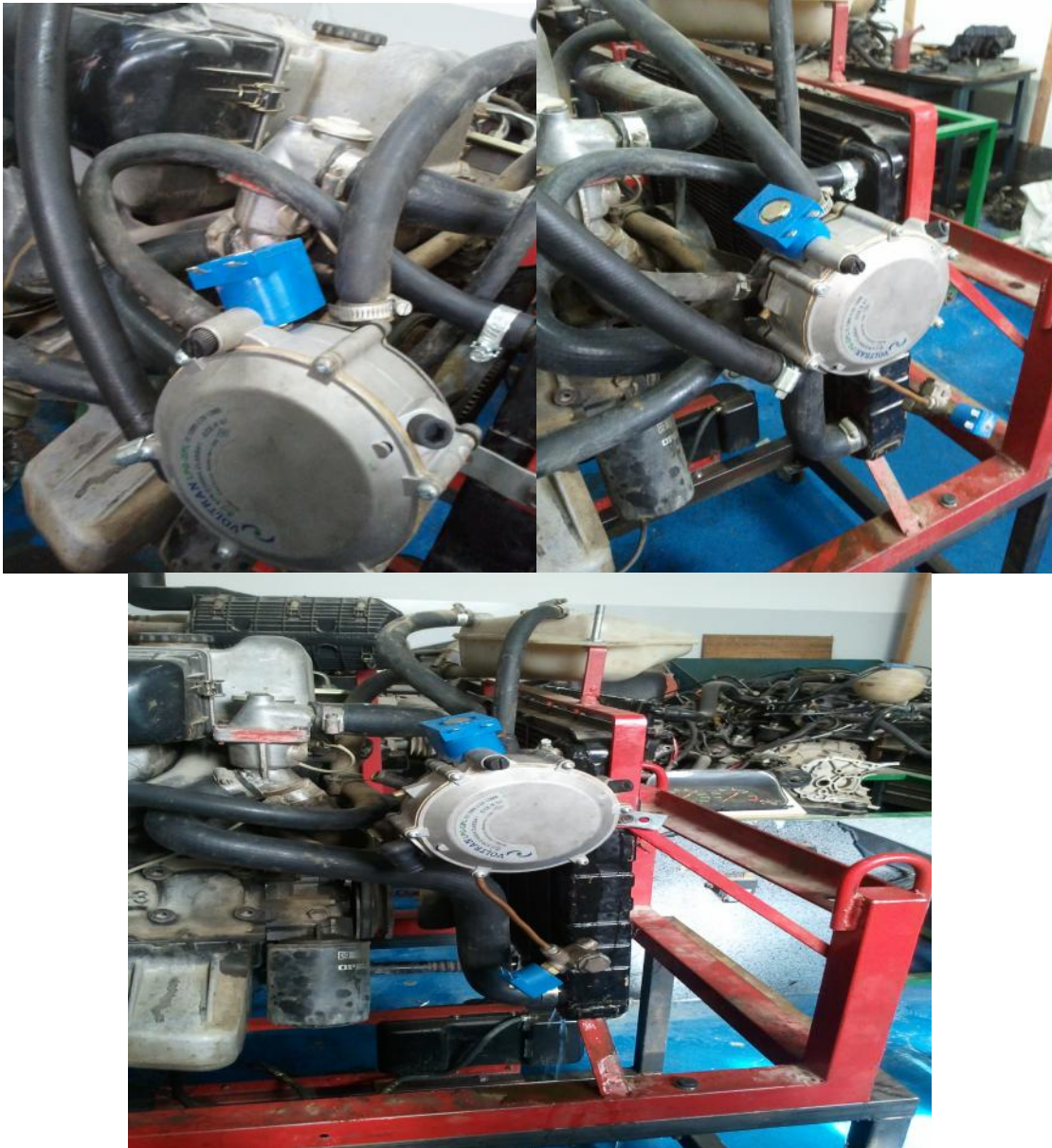
Figure (5-11): Fixing evaporator
