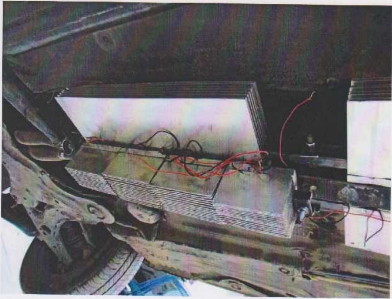
Figure 6.2: Ready TEG system installed at the vehicle.
