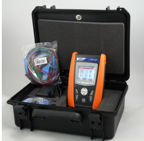
Fig.4.1. Vega 78 power quality analyzer device .
