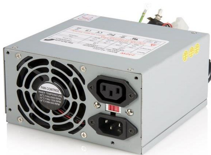
Figure (4.8): Power Supply
