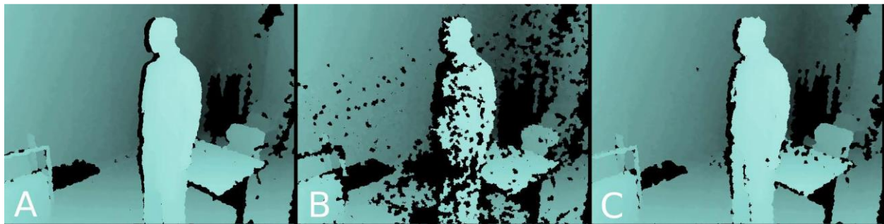
Figure (4.5):Multi Kinect sensors depth data
