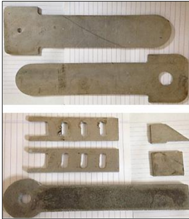
Figure 3 32: The machined parts using Plasma CNC
