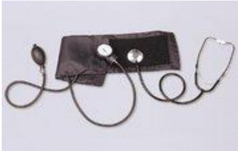
Figure 3.10 Auscultatory method aneroid sphygmomanometer with stethoscope [14]
