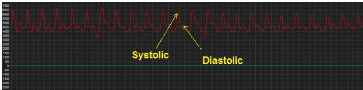
Figure 5.10 Signal after Ac coupling and filters
