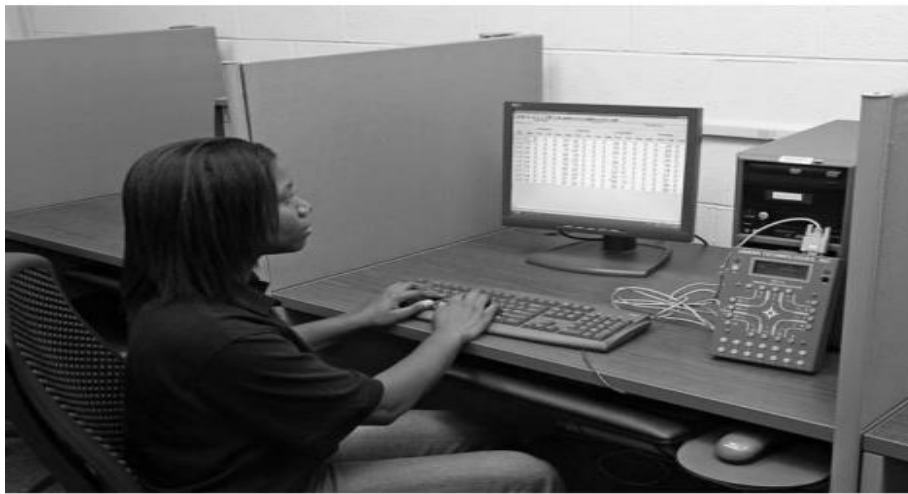
Figure 3-1 Traffic Data Collector TDC-12 Hooked to a Computer.
