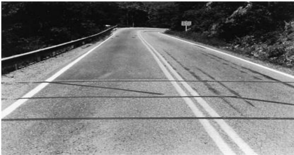
Figure 3-2 A Sensor Setup of a Surface Detector Using Pneumatic Road Tube
