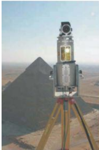
Figure (3-8): LMS-Z420i with calibrated high-resolution digital camera Nikon D100 at the top of the Cheops Pyramid, Egypt [14]
