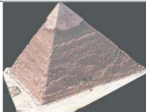
Figure (3-10): Single scan from the north and east faces of the Chephren Pyramid visualised as a coloured point cloud.[14]
