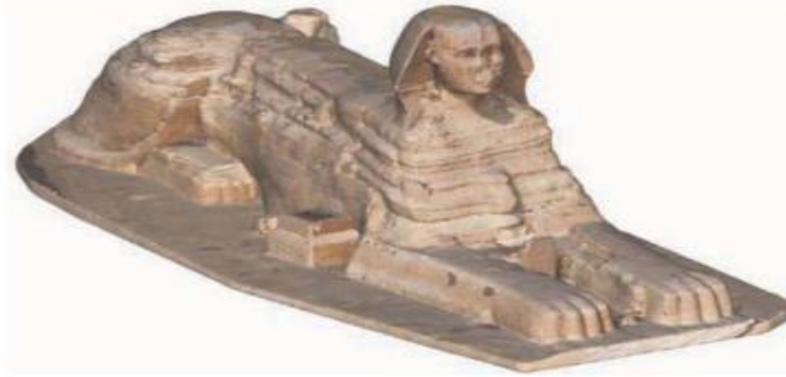
Figure (3-11): Triangulated point cloud of the Sphinx textured in Rican Pro, combined from seven scanner positions: six from the ground and one from the Cheops Pyramid.[14]
