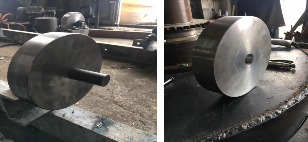
Figure 3.5: Pulleys of tank
