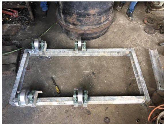
Figure 3.4: Base of tank
