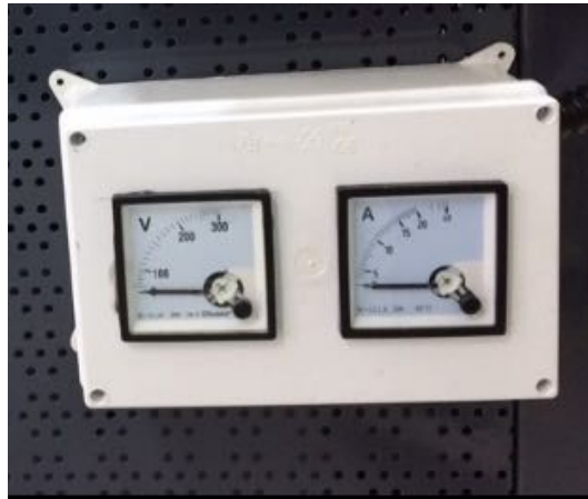
Figure 4.8: Ammeter and Voltmeter
