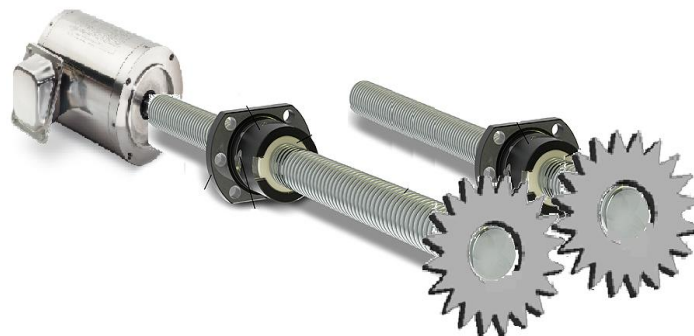
Figure 3.4: The screw tied nut and gear connect with motor for width
