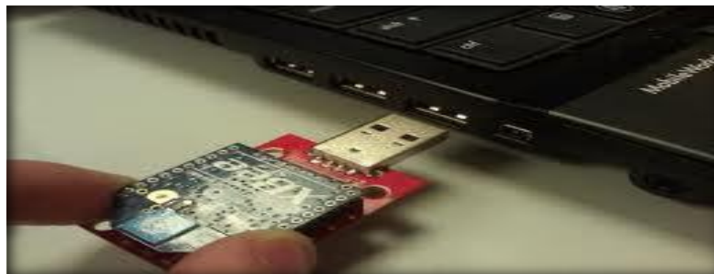
Figure 6.2: XBee connected to computer using dongle.
