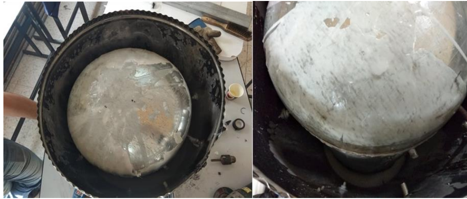
Figure (3.10) PW at Liquid State Insert Around Hot Water Tank
