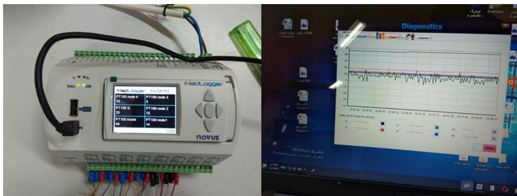
Figure (3.11) PT100 Sensors Connect to Data logger
