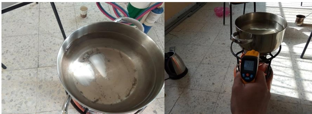
Figure (3.9) Dissolved PW Using Flame Source Above Melting Point (60-62 °C)
