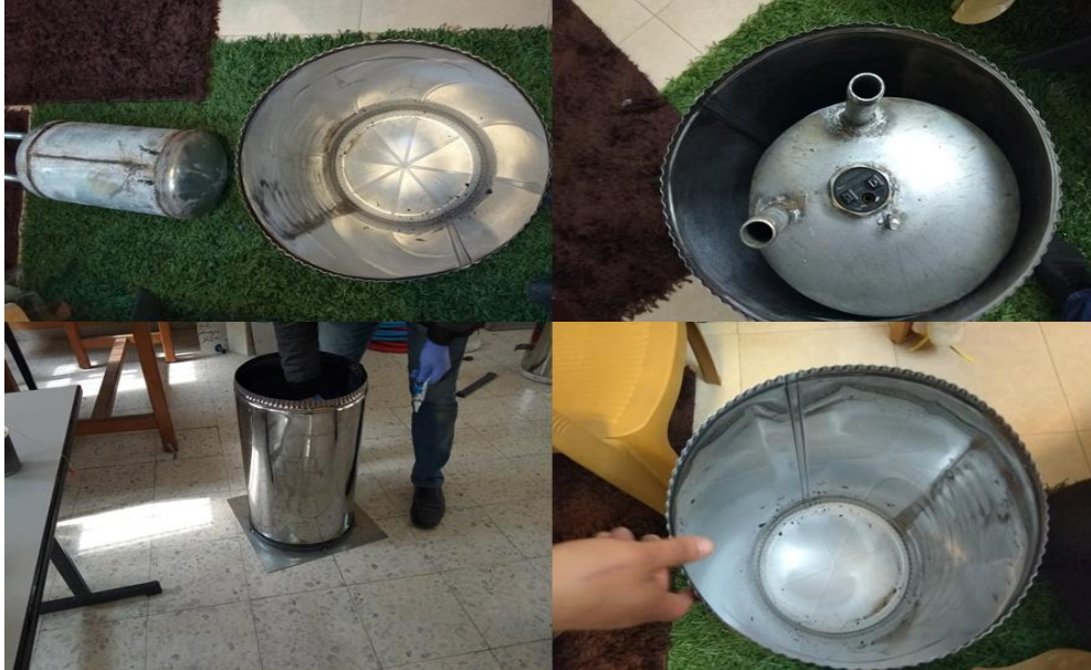
Figure (3.7) Preparation HWST Using PW Walls
