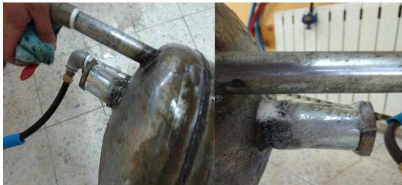
Figure (3.5) HWST Leaking Test
