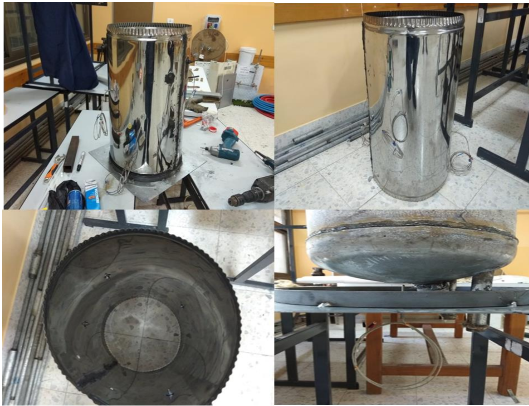
Figure (3.8) Fixed PT100 Sensors in HWST Design Using PW
