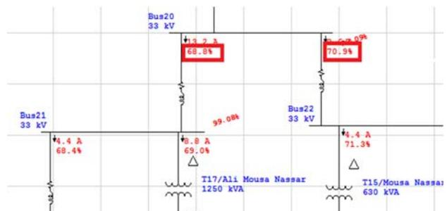
**Fig. 6. Power factor for industrial load feeders**
