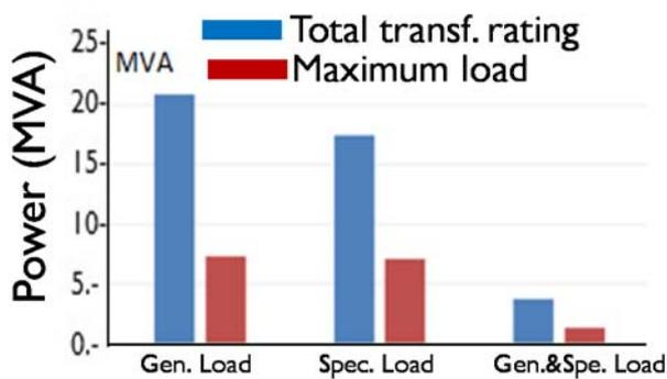
Fig. 1: Maximum load and transformers rating for each load category.
