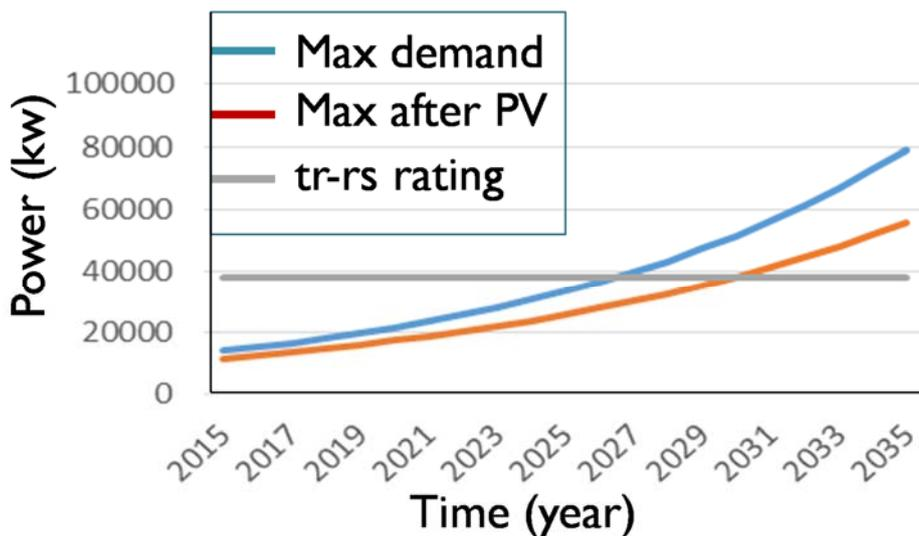
Fig. 11: Maximum demand before and after installing PV system.
