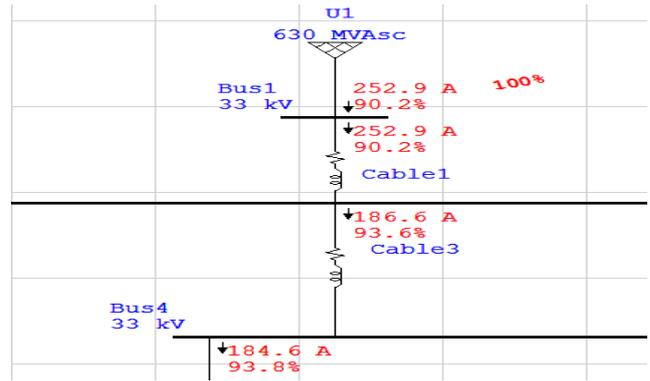
**Fig. 5. Maximum current at interconnection point for present case**
