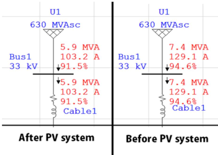
Fig. 10: Interconnection point state before and after adding PV system.
