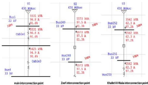
Fig. 8: Interconnection points after installing capacitor banks.
