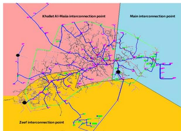
**Fig. 7.: Yatta's medium voltage scheme after adding 2 interconnection points.**
