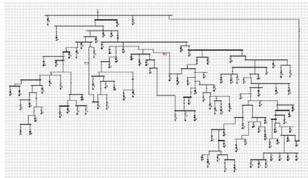
Fig. 3: Single Line Diagram for Yatta city using ETAP Software.
